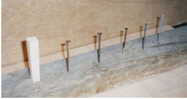
Photo 2.41: Different materials used to make nails.
