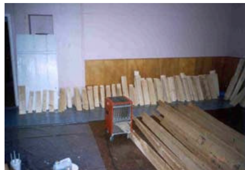
52. New shingles: The shingles were dried in room temperature (+25°C). Moisture was monitored during the drying period.
