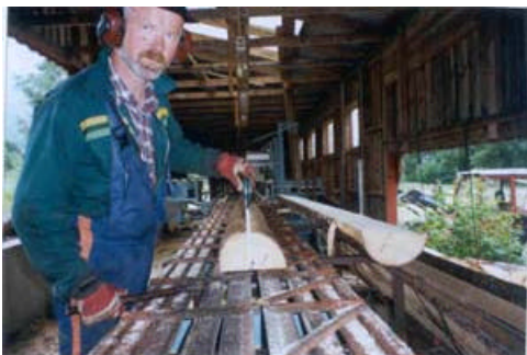
51. New shingles: Standing spruce trees were selected during sap time. The trees had been growing very slowly. The shingles were cut perpendicularly.
